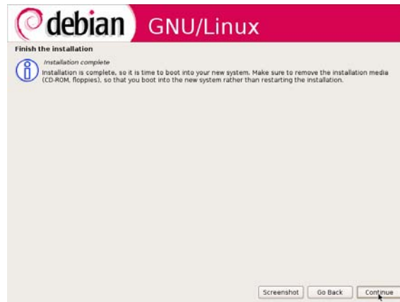
Gambar 2.54 Finish the installation
